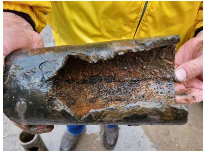
Photo DW&FP-1: Domestic Cold Water Pipe Break Near Housing Unit No. 6
